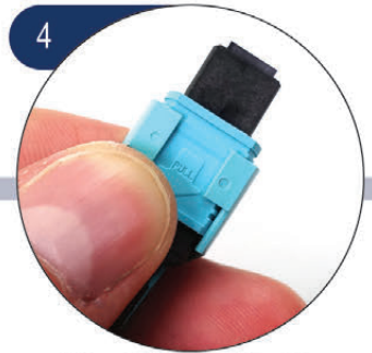
4 When fully rotated the tab will snap in place
