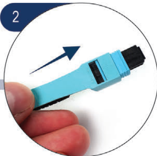
2 Slide tab forward over MPO rear body until it snaps in place
