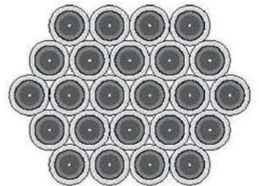
2.0mm Diameter Cable 24 Fiber Bundle
